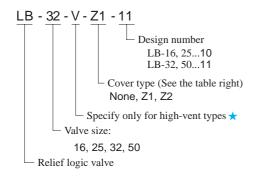
★ Use high-vent pressure types if the shifting time from unloading to on-loading is reduced.
